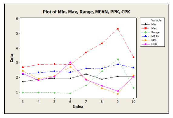
Here we can clearly see that the dwell time is also a key factor in capability and beyond a certain point increases the peel strength but also increases the Standard Deviation and range so losing capability.
