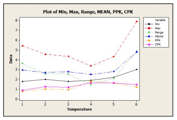
Above we can see the effects of temperature, what this revealed was that temperature did not have a big effect on process capability, however high temperature did result in higher peel strength values.
