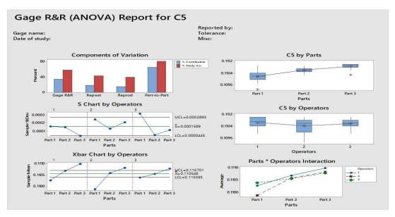
As you can see, way too much variation in the measurement. This was caused by the fixturing of the part on the inspection system. If the part is not at 90 degrees to the
